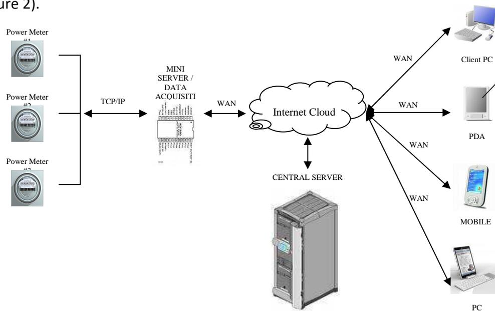
Figure 2 - PQ Monitoring System
