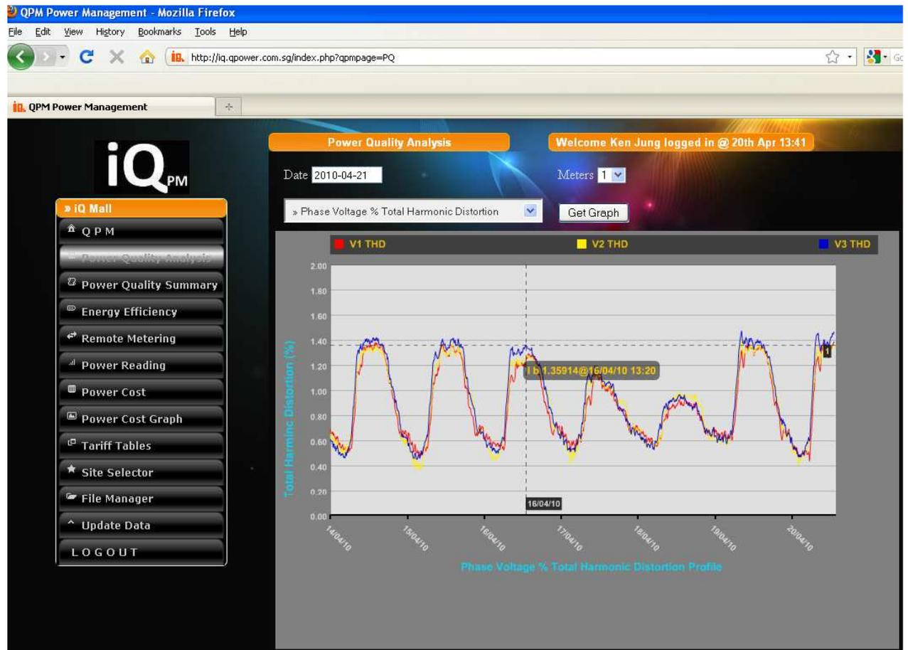
Figure 5 – Phase Voltage % Total Harmonics Distortion Profile
