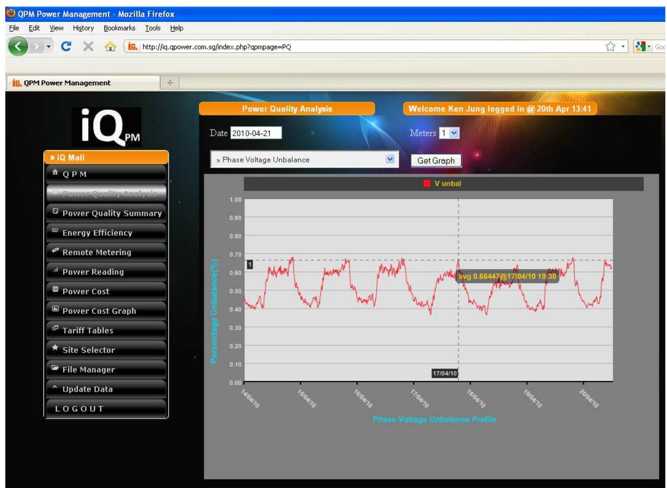
Figure 4 – Phase Voltage Unbalance Profile
