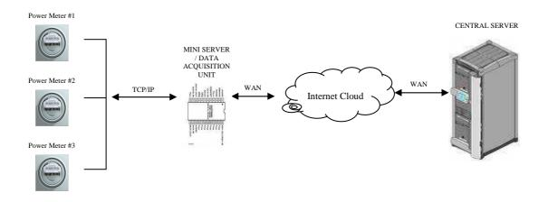
Figure 1 - iQpm system: Data acquisition (iQpm-DA) Unit & the PQ analyzer (iQpm-PQA) Unit
