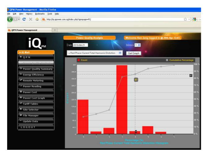
Figure 8 – Red Phase Current Total Harmonic Distortion Histogram
