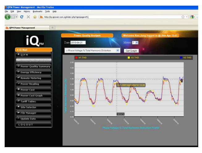
Figure 5 – Phase Voltage % Total Harmonics Distortion Profile
