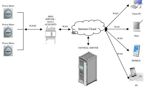
Figure 2 - PQ Monitoring System
