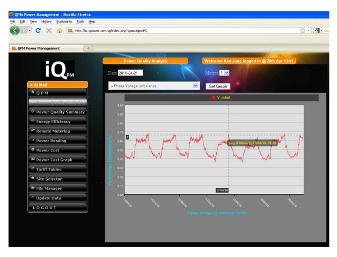
Figure 4 – Phase Voltage Unbalance Profile
